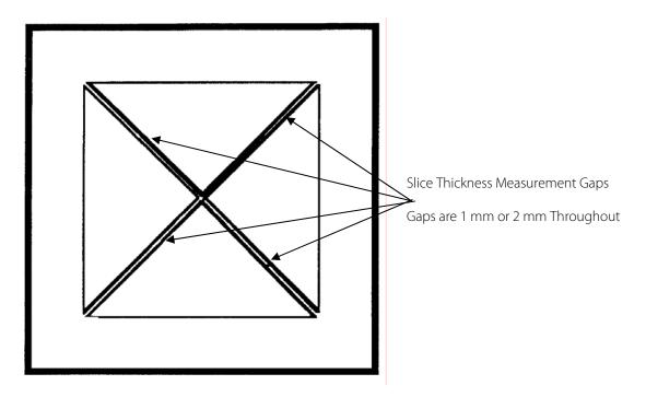
Figure 1-5. Slice Thickness Sections
